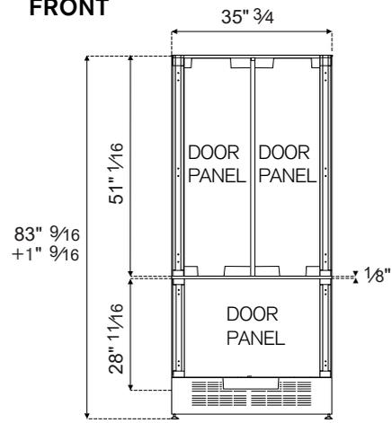
+1" 9/16 for the adjustable max height of the leveling feet
