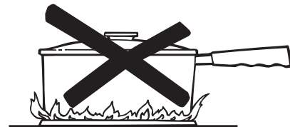
These flames are too large for the pot
