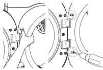
**9** Insert the latch on the right side and install the latch screws.
