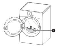
Always ensure that the lint filter is properly installed before running the dryer. Running the dryer with a loose or missing lint filter will damage the dryer and articles in the dryer.
