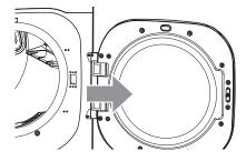
7 Move the door to the left side and line up the holes in the hinge with the holes in the cabinet.
