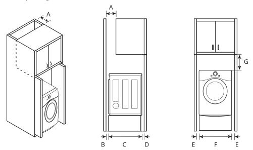
For cabinet installation with a door, minimum ventilation openings in the top of the cabinet are required.
