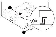
3 Preassemble a 4" (10.2 cm) elbow S to the next 4" (10.2 cm) duct section, and secure all joints with duct tape. Be sure that the male end of the elbow faces AWAY from the dryer. Insert the elbow/duct assembly through the side opening and press it onto the adapter duct. Secure it in place with duct tape. Be sure that the male end of the duct protrudes 1.5" (3.8 cm) to connect the remaining ductwork. Attach the cover plate S to the back of the dryer with the included screw.
