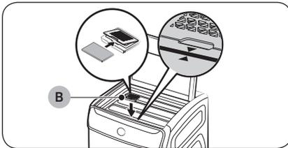
3. Insert a folded dryer sheet in **dryer-sheet case (B)**, and then put the case at the top center of the rack. Make sure the dryer-sheet case faces against the triangle mark on the upper dryer because only the arrow area has the built-in magnet to secure the filter.
