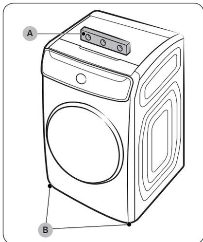
Using a **level (A)**, check if the dryer is level side to side and then front to back. If the dryer is not level, turn the **leveling legs (B)** clockwise to lower the dryer or counterclockwise to raise the dryer.
