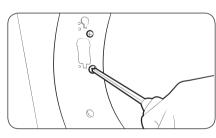
8. Re-insert the two screws that held the lever holder into the same screw holes, and then tighten.
