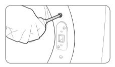
13. Re-attach the remaining screws to the remaining holes above and below the lever holder, and then tighten.
