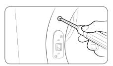
**6.** Remove the two screws above and below the lever holder on the opposite side of the door opening.
