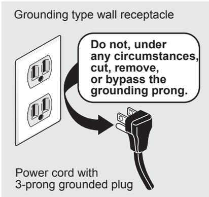
**CIRCUIT** - Individual, properly polarized and grounded 15 amp. branch circuit fused with 15 amp. time delay fuse or circuit breaker.
