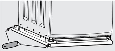
3. With help from a second person, carefully tip the laundry center slightly to the left as shown in the picture below. Remove the foam shipping support from the base of the unit. Save packaging foam for future use.
