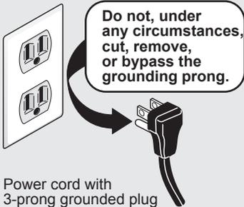
1. The laundry center is equipped with a three-prong (grounding) plug for your protection against shock hazard and should be plugged directly into a properly grounded three-prong receptacle.
