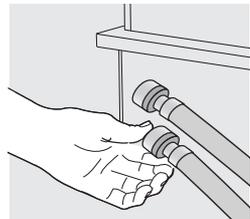
Tighten by hand until snug. Then tighten each supply connection another 2/3 turn with pliers. **DO NOT cross thread or over-tighten these connections.**
