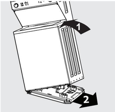
4. Carefully lower the laundry center to an upright position and remove the tape holding the lid shut. Remove the foam tub block, all foam inserts, and other tub contents.
