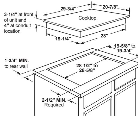
To ensure accuracy, it is best to make a template when cutting the opening in the counter
