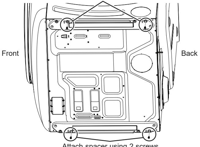
Attach spacer using 2 screws
