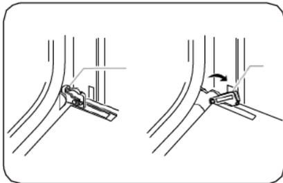
A. Oven door hinge lock locked position
