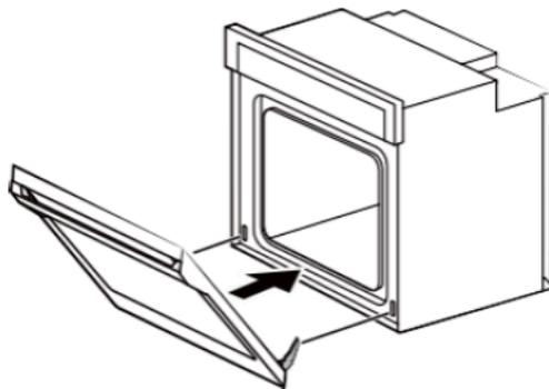
1. Using two hands, grasp side edges of door at the midpoint. Face the oven cavity.
