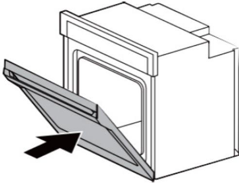
4. Lower the oven door to the fully open position. If the oven door does not open to a full 90°, repeat steps 1 through 3.
