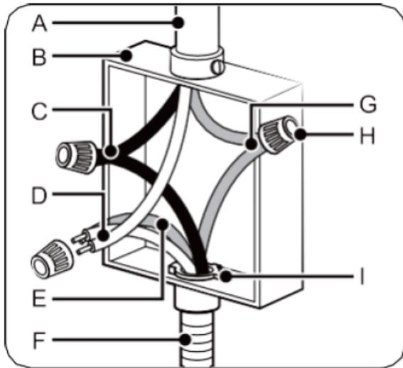
1. Connect the 2 black wires (C) together using a UL listed wire connector.
