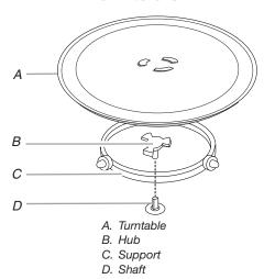
The turntable can rotate in either direction to help cook food more evenly. For best cooking results, do not operate the microwave oven without having the turntable in place. See the "Assistance or Service" section to reorder any of the parts.
