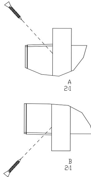
4. Secure trim kit frame to cutout/cabinet by installing four long wood screws (painted) into the pilot holes drilled in Step 3 above.
