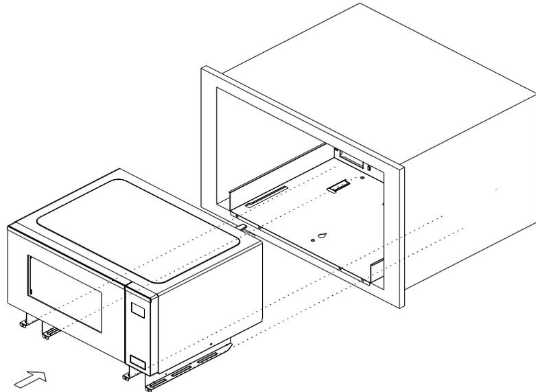
4. Secure the microwave oven to the cutout/cabinet by installing four 123# screws into the mounting holes.
