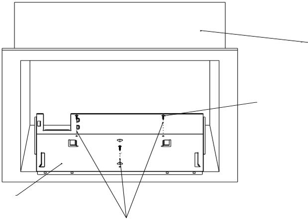
A. Bottom duct mounting holes C. Bottom duct
