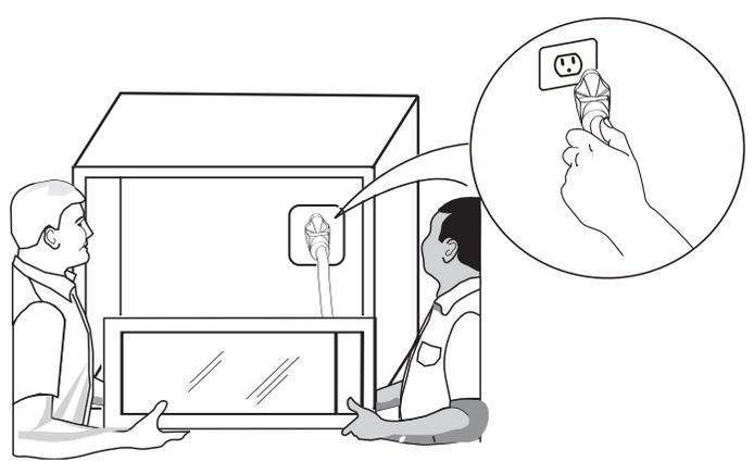
3. Slide the microwave oven back and into place. The mounting holes of the rail flanges and bottom duct flange will align against the bottom front facing of the cutout/cabinet opening.
