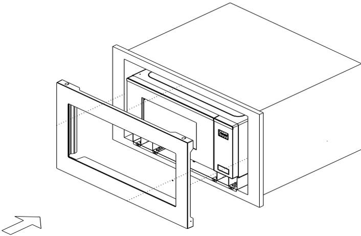
2. To vertically center the trim kit frame, slide it upward, against the opening, until the upper tabs catch against the top of the rails.
