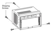
2 Slide the unit from the cabinet by gripping the base pan handle and pulling forward while bracing the cabinet.
