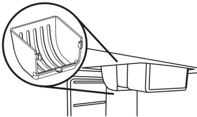
3. Replace bulb with a 40 W maximum appliance bulb or an LED bulb rated for wet/damp locations.
