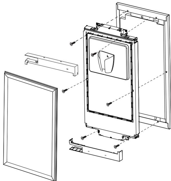
6. Snap the upper and lower trims back on the inner panel.
