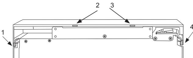
3. Pry on each tab and pull down on the trim as shown until you can remove each of the trims.
