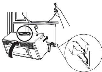
**NOTE:** When mounting the microwave oven, be careful of the damper not be damaged by wall or cabinet.
