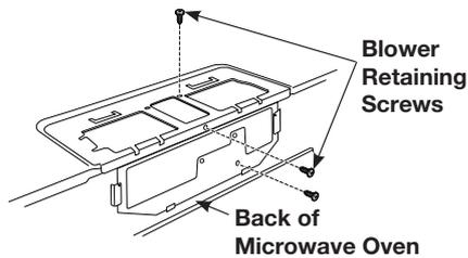
2. Open the blower door by lifting it up at the back of the microwave. Remove and save the blower shield on the back of the microwave by sliding it up.
