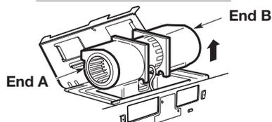
**CAUTION:** To avoid breaking or cracking the blower blade, do not touch the blade. Hold the outer case of the blower when you pull it out or put it back in place.
