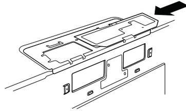
8. Secure the blower to the microwave using the blower retaining screws from Step 1.
