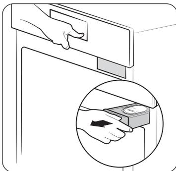
1. Locate the water reservoir. The water reservoir is on the right side of the oven, just above the oven opening. Touch **Open/Close Reservoir** on the control panel to eject the water reservoir. Grab the front of the reservoir, and then slide it out to remove.
