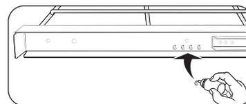
5. Repeat for the right (front and back) slide mechanism of the rack.
