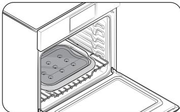
4. Push the container in until the steam nozzle enters the hole on the convection fan cover.
