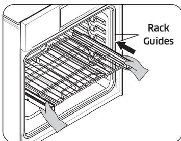
With the Gliding rack in the Closed position and the oven off, carefully insert the Gliding Rack between the guides until the rack reaches the back.
