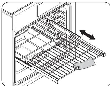
When using the Gliding rack in the oven, be sure to pull on the handle of the rack only to slide it in and out. If you grasp the frame while using the rack, the entire Gliding rack will be removed. Make sure you use oven gloves when handling the Gliding rack during cooking.
