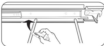
3. If there is debris in the slide tracks, wipe it away using a paper towel. (Any graphite lubricant wiped away must be replaced - See steps 4 through 7).
