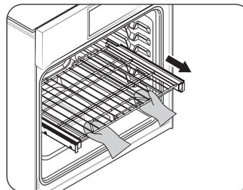
With the Gliding rack in the Closed position and the oven off and cool, grasp the rack and frame and pull both forward to remove.
