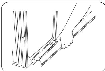
1. Using two hands, grasp the side edges of the door at the midpoint. Face the oven cavity.
