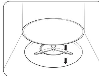
Remove all packing materials inside the oven. Install the roller ring and turntable. Check that the turntable rotates freely.
