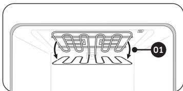
2. While holding the glass cover with one hand, insert a flat-sharp tool such as a table knife between the glass and the frame to remove the glass cover.
