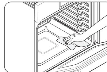
6. Clean the oven's interior. There will be a significant amount of water remaining on the bottom after a steam-cleaning cycle. Remove the residual water with a sponge or soft dry cloth.
