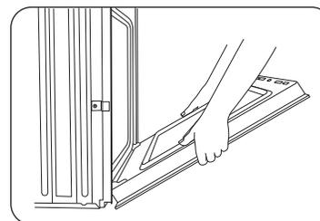
4. Lower the oven door to the fully open position. If the oven door does not open to a full 90 °, repeat steps 1 through 3.
