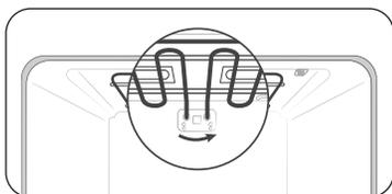
1. To change the halogen bulb, you must tilt the broil heater down. To do this, turn the circular nut on the support counterclockwise while holding the broil heater. The broil heater should loosen and tilt down.
