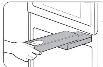
3. Replace the cap or the clear plastic top, and then slide the water reservoir back into the reservoir slot.
