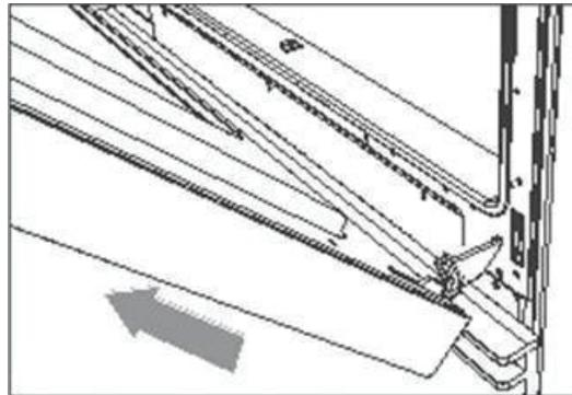
2. Open the levers fully on both sides.
