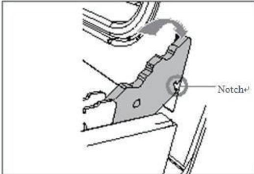
2. Insert the hinge tongues into the slots making sure that the notches on both sides drop into place as shown.
