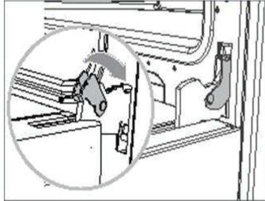
4. Fully close the levers on the left and right hinges, as shown, then close the door.
