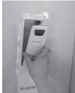
5. Push bulb cartridge down onto mount.
