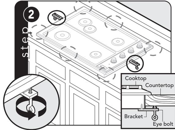
Screw the eye bolt into the self-retaining nut and tighten firmly against bottom of countertop.
