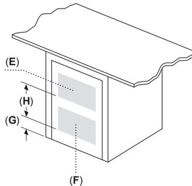
If the front of the appliance is covered, louvered openings must be installed as shown and front/rear clearances adhered to according to closet installations.
